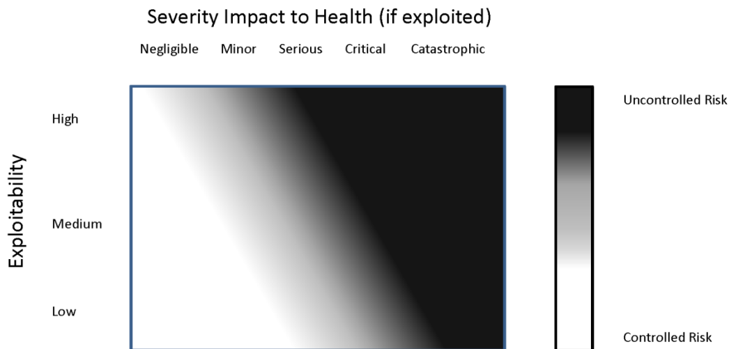
Figure – Evaluation of Risk to Essential Clinical Performance. The figure shows the relationship between exploitability and risk to health, and can be used to assess the risk to the device’s essential clinical performance from a cybersecurity vulnerability. The figure can be used to categorize the risk to essential clinical performance as controlled or uncontrolled.
